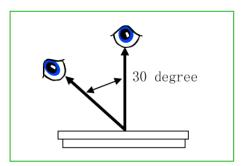
Under daylight lamp 20 $\sim$ 40W, product distance inspector 'eye 30cm,incline degree 30°  $_{\circ}$
