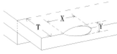
$\Phi = (x+y)/2 > 2.5 \text{ mm}$<br>Reject                                                                                                                 |
