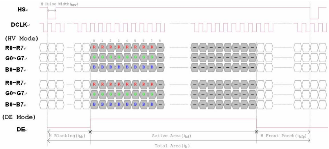
Horizontal input timing diagram
