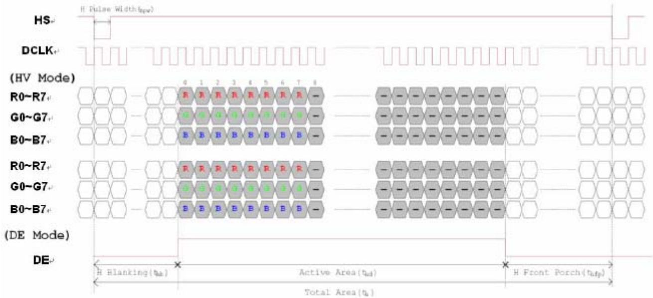
Horizontal input timing diagram
