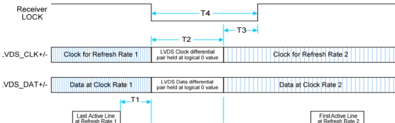
T1 - Min delay from start of vert blank to start of timing change: 2 lines (HSYNC periods)
