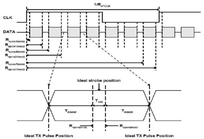
T<sub>RSKM</sub>: Receiver strobe margin R<sub>SPOS</sub>: Receiver strobe position T<sub>SW</sub>: Strobe width (Internal data sampling window)
