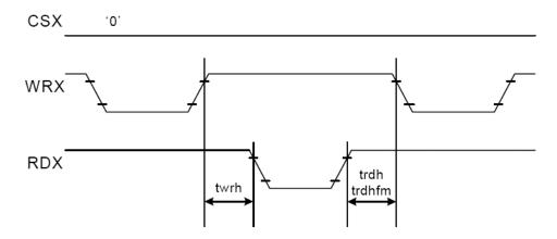
Note: Logic high and low levels are specified as 30% and 70% of VDDI for Input signals.
