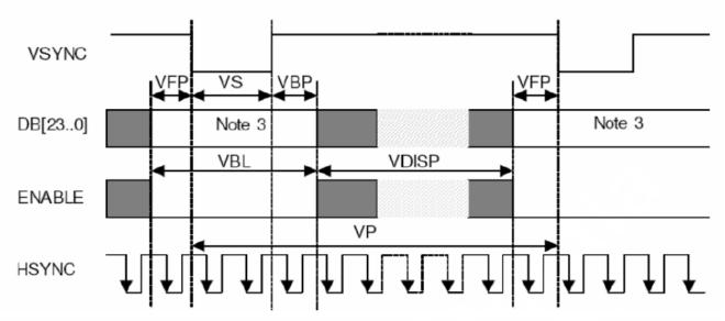
(Resolution=480x854, VSSA=VSSD=0V, VDD1=1.65V to 3.3V, VDD2=2.5 to 3.3V, VDD3=2.5 to 3.3V,  $T_A = -30$  to  $70 \,^{\circ}\text{C}$ )
