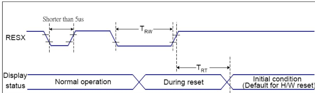
Figure 9 Reset Timing
