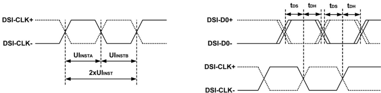
Fig. 7.1.1 DSI clock channel timing
