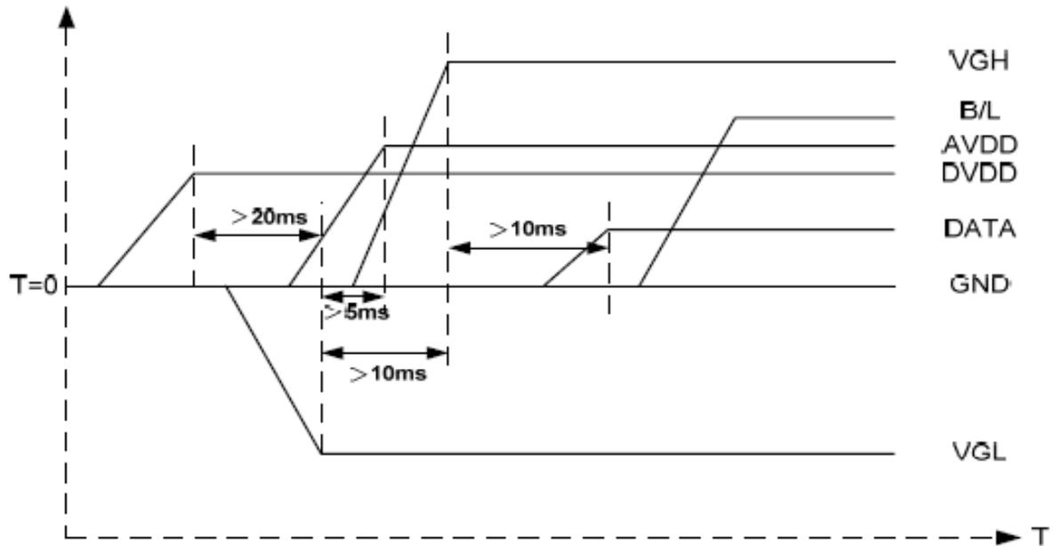
**DV<sub>DD</sub> → VGL → VGH → Data → B/L**
