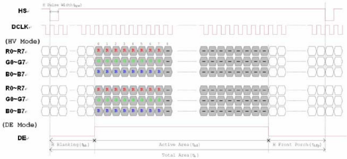
Horizontal input timing diagram
